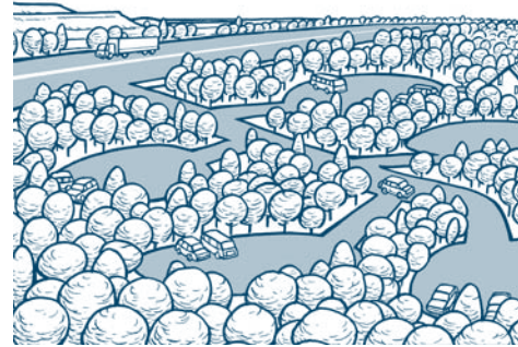
A single continuous zone has a more imposing presence in the landscape than solutions where parking areas are fragmented and spread out.
