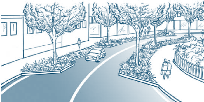
The narrowing of the road and the appropriate landscaping treatment on the margins (the introduction of trees for example) will have the effect of slowing down the traffic.
