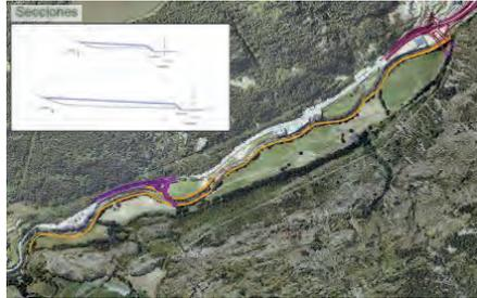
*Figure 18: Orthophotograph of the area concerned by the project; the mouths of the two parallel tubes are visible, as are the roundabouts forming the junction with the existing road. The canalised area is shown in orange and behind this the area where the excavated stones and earth are to be deposited. The sections show how the material is positioned*
